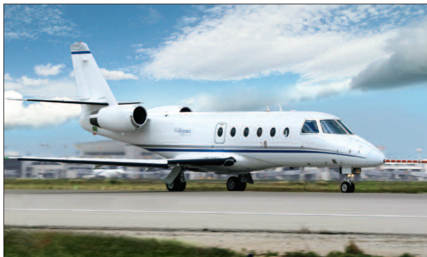
Similar to the G100, the G150's fuselage is built from cross-sectional frames, longerons and stressed skins, but it's stretched 16 inches aft of the wing to balance the weight of the wider and heavier fuselage.
