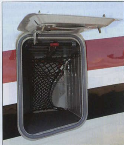
There is a small aft, external compartment that will hold up to 77 pounds of baggage.
