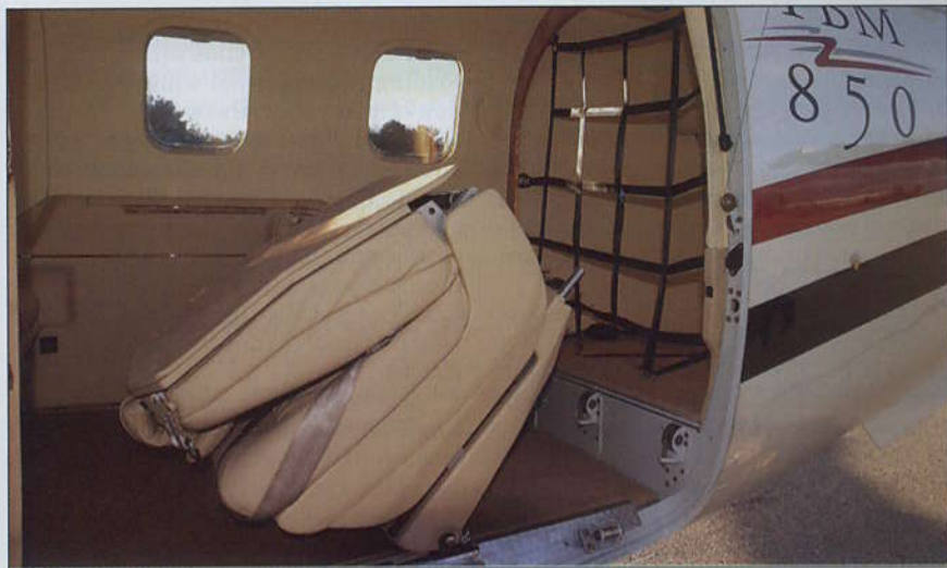
The aft baggage compartment in the cabin can accommodate up to 220 pounds of luggage.
