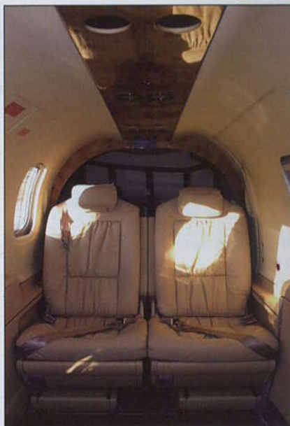
The passenger seats measure 18 inches wide with 22-inch-high backrests.
