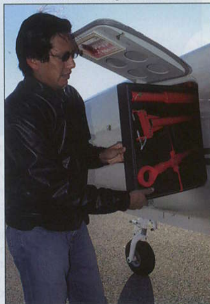
A separate, forward compartment holds the collapsible tow bar and duct covers.
