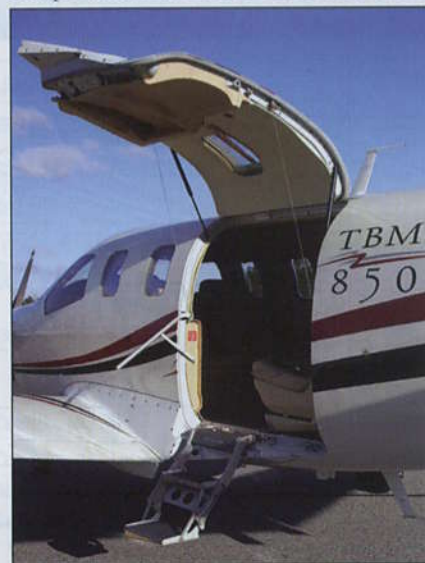
A swing-down boarding ladder and a sturdy handrail make it easy to climb aboard the aircraft.
