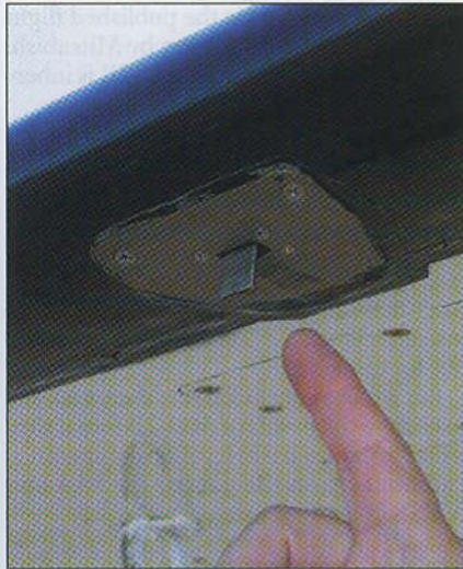
The stall detector on the right-wing leading edge is linked to the stall-warning stick shaker.
