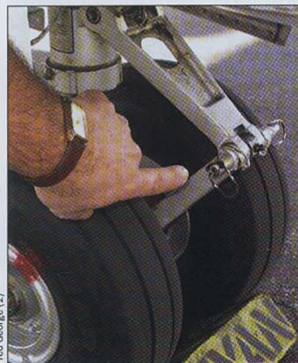
Nosewheel steering linkage must be disconnected for towing. Don't forget to replace the quick release pin in the scissors link before start.
