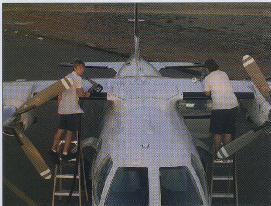
Crownair's Devin Funderburg and Greg Scott refill the main tanks. The aux tanks and tiptanks must be refilled separately, if needed. Pilots need to check all six fuel caps on preflight inspection.
