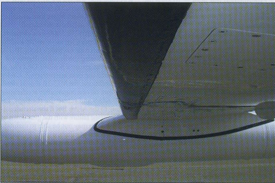
The wings are relatively short and thin. Twin tip tanks that feed the main 154 gallon (1,032 pound) wing tank increase fuel capacity by 180 gallons (1,206 pounds). Aux wing tanks, outboard of the engines, add another 69 gallons (462 pounds) for a total usable capacity of 403 gallons (2,700 pounds).
