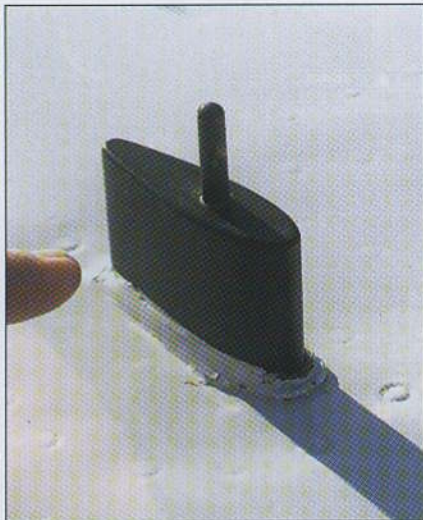
An optional ice detector is a must, in our opinion. It provides the crew timely warning about impending ice accretion so that ice protection systems can be used effectively and an exit strategy can be executed.
