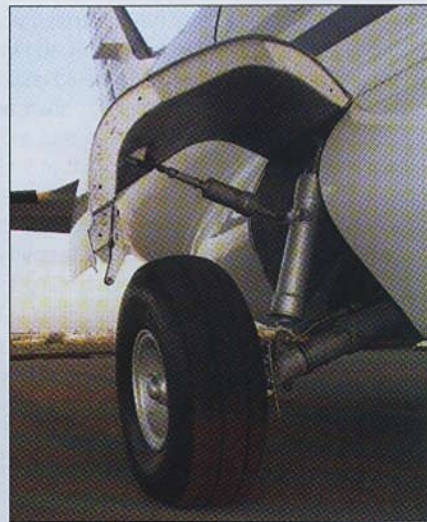
The main landing gear are beefy, well-suited for rough field operations. On long-body models, they're positioned 16-inches aft of the c.g.
