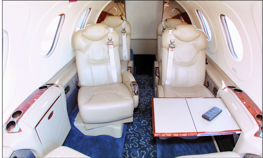
The cabin has three windows on each side, mounted for eye-level viewing from the seated position. Dual cup holders, air outlets and reading lights are provided for each seat. An overhead light also is provided for each foldout work table.
