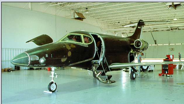
While it is still undressed, you can see the extensive use of composites.
