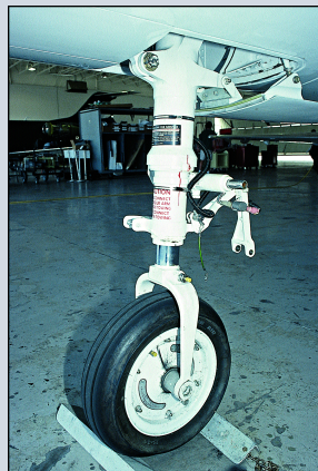
The nose gear of the Premier includes a fully detachable link for 360-degree taxiing and a nose-gear squat switch.
