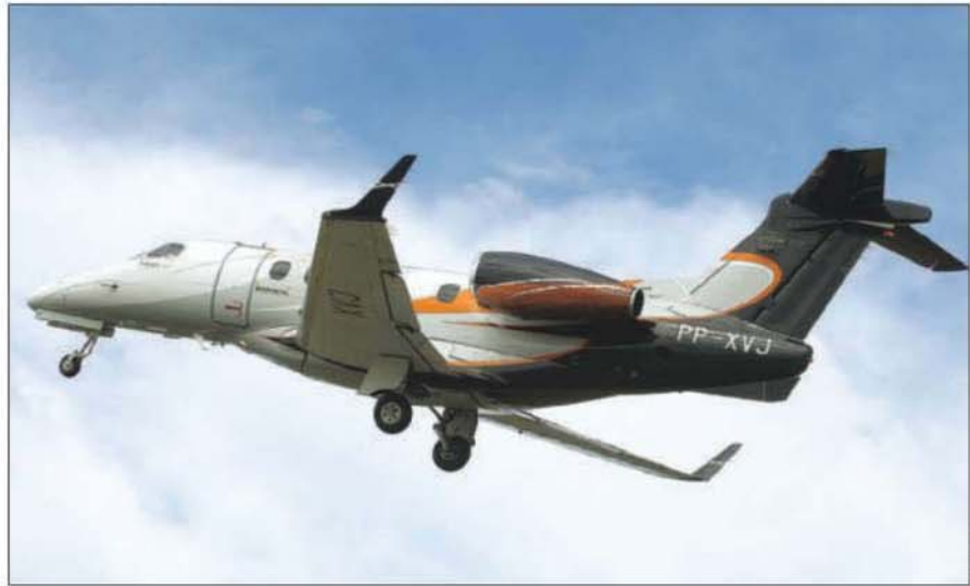
Climb performance is impressive. The aircraft can depart at MTOW, climb directly to FL 450 and then cruise at 370-plus KTAS while burning 840 pph.
