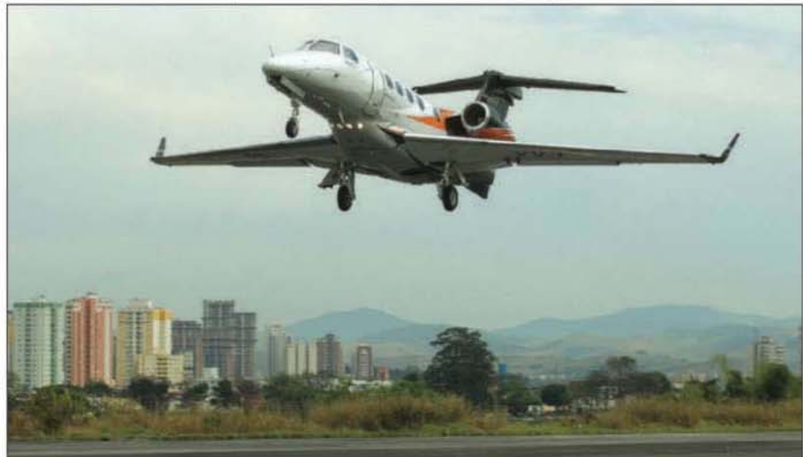
Phenom 300's climb performance is impressive. The aircraft can depart at MTOW, climb directly to FL 450 and then cruise at 370-plus KTAS while burning 840 pph.
