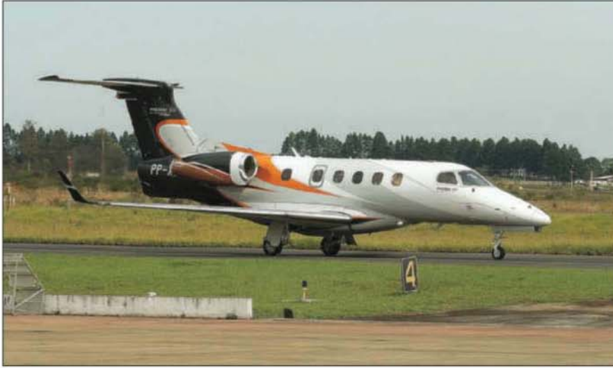
The Phenom 300 features brake-by-wire with high-capacity carbon heat packs. Pedal pressure, similar the Embraer's jetliners, is heavy but braking action is very smooth.
