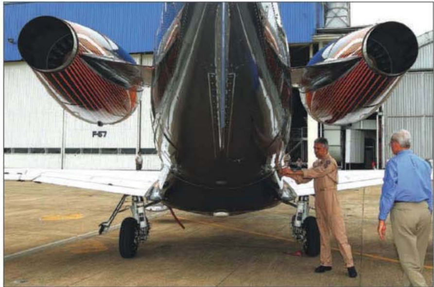
The Phenom 300 is designed for easy access to systems and high-frequency utilization, similar to Embraer's jetliners. The design expedites the crew's preflight inspections.
