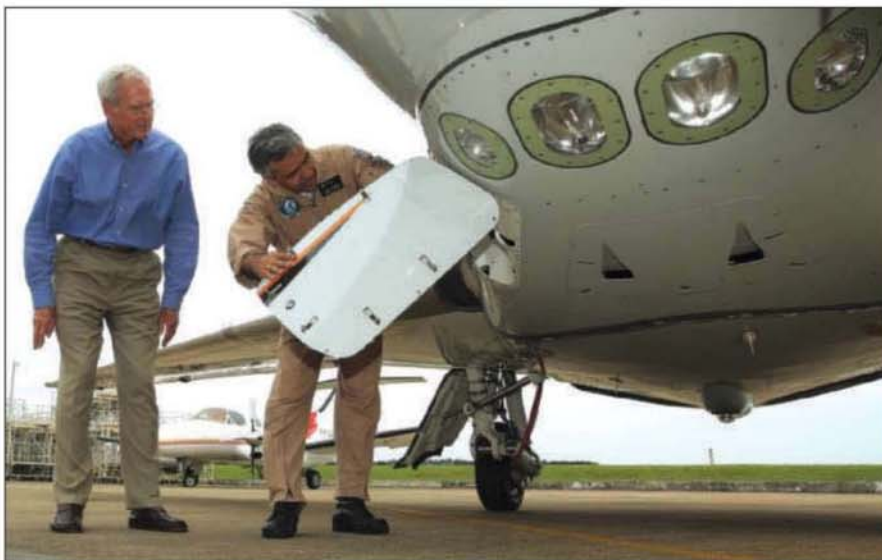
Capt. Eduardo Menini opens the single-point pressure refueling access door ahead of the right wing. The SPPR panel has LED illumination for night operations and a selectable refill quantity feature.
