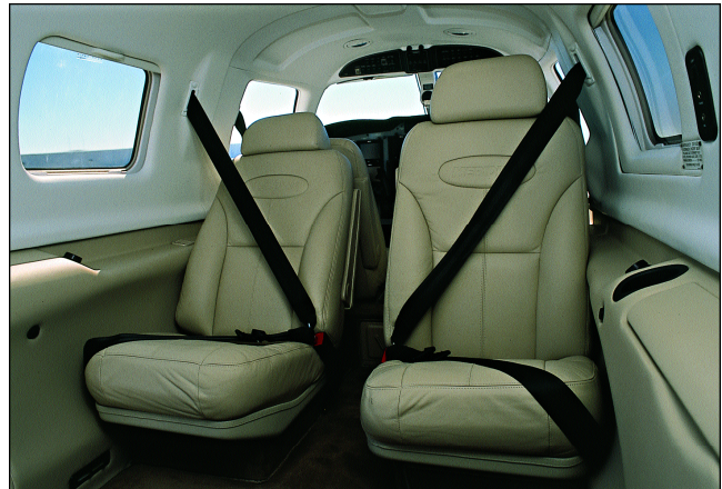
To enhance the sense of spaciousness, most of the interior edges are rounded.
