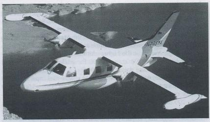
Mitsubishi Aircraft International's new model Marquise incorporates two 1,000-shp. Garrett AiResearch TPE331-10-501M turboprop engines flat-rated to 715 shp. The Marquise can be distinguished from its predecessor, the MU-2N, by a smaller diameter tailpipe exhaust, and from the smaller Solitaire by the lower side bulges housing the main landing gear.
