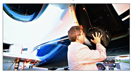
The 240-cubic-foot external baggage compartment, with Class C fire protection, also is accessible through a door in the aft cabin.
