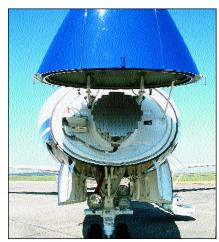
The radome accommodates a 10-inch weather radar antenna.
