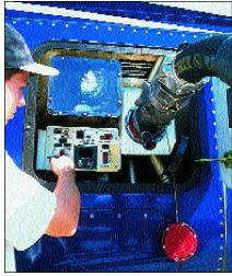
All walk-around preflight tasks can be done with feet on the ground, including refueling.
