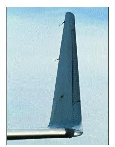
Winglets and auxiliary fuel tanks boost range to 3.200 nm.
