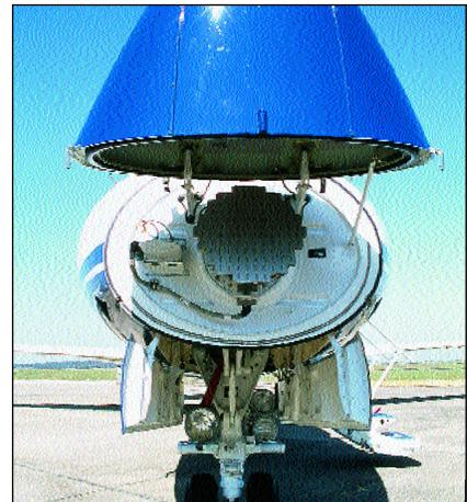
The radome accommodates a 10-inch weather radar antenna.
