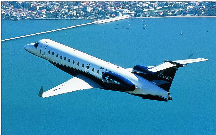
Docile slow-speed handling characteristics and low  $V_{REF}$  speeds make Legacy easy to fly in the pattern.
