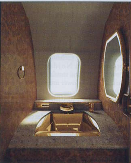
The lavatory has been redesigned to expose the cabin window on the left side of the compartment.
