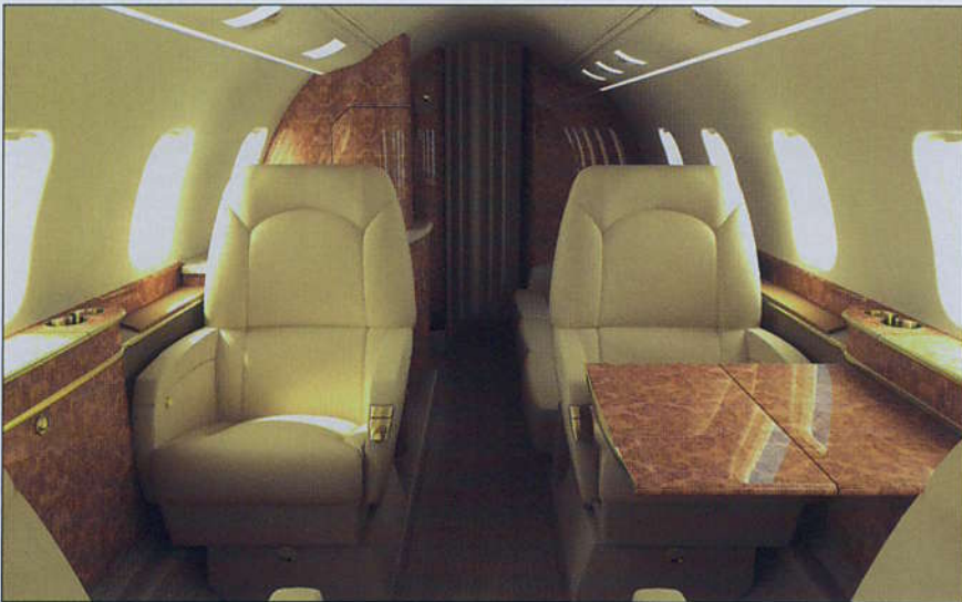
LED lighting replaces the overhead fluorescent wash lights and reading lights.
