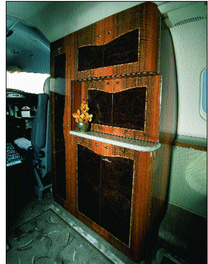
The refreshment center's ice-chest drain requires aircraft electrical power to drain off water accumulation. Operators say this quirk is an inconvenience during overnight layovers.
