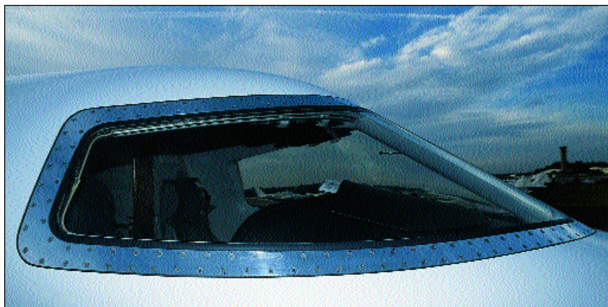
Glass-faced windshields, a first for a Learjet, have been prone to cracking and optical distortion. A change in the tempering process is supposed to remedy the problem.
