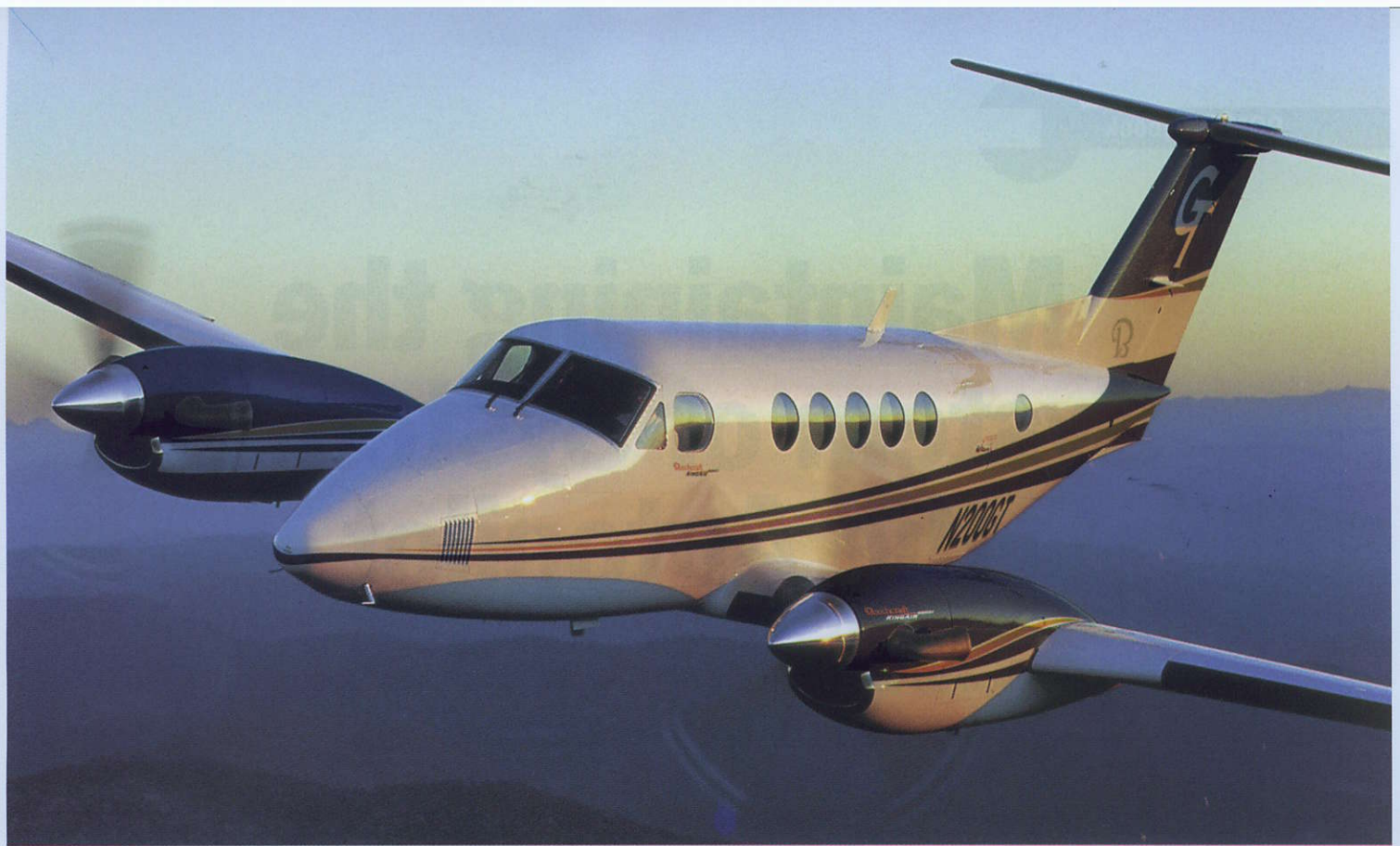
Beech opted for a T-tail empennage with swept vertical and horizontal surfaces. The configuration keeps the horizontal stabilizer out of the prop wash to reduce vibration and its high, aft position improves aerodynamic effectiveness.
