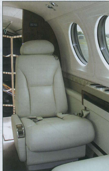
Each chair has an aisle-side armrest. The other armrest is built into the sidewall, resulting in 18 inches of net seat width. Seat cushions are 20 inches long, providing good thigh support. Seat backs are 28 inches tall, including headrests.
