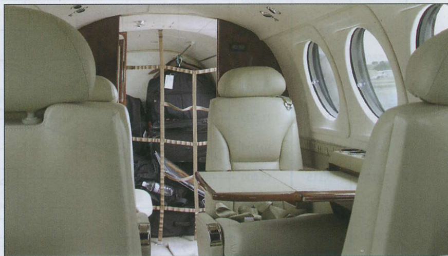
Sturdy 23-by-22.5-inch worktables are enclosed in side pockets between the facing chairs of the club seating section. AC power outlets are provided on both sides of the club section.
