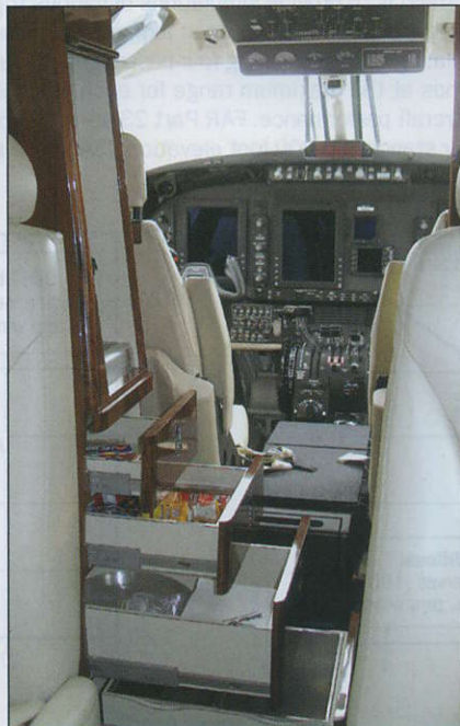
A refreshment center located behind the cockpit bulkhead has a water tank, heated beverage container with overboard counter drain, two cup dispensers, three storage drawers and a double ice chest drawer.
