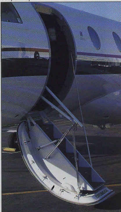
The Jetstream 41's counter-sprung airstair door is easy to open and close.
