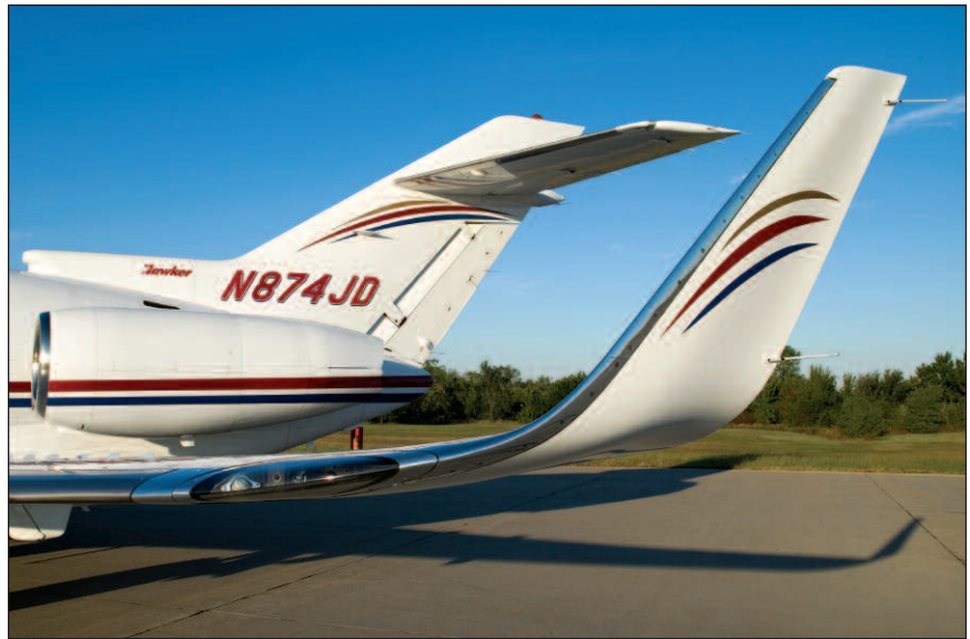
Raytheon's homegrown winglets add about 4 percent or 100-nm range. In addition, their design is consistent with the Hawker 850's extended 600-hour scheduled maintenance intervals.
