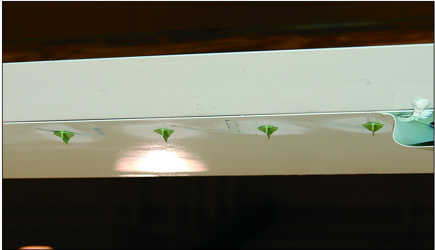
Aerodynamics is a black art as much as a science. V-shaped wave generators on the tail have been removed in favor of ultra-low-profile, fin-shaped vortex generators.
