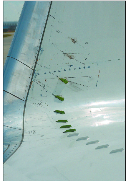
At the highest cruise speeds, sonic flow "hot spots" form at certain sections of the aircraft, creating shock-induced separation. Fin-shaped vortex generators energize the boundary layer, thus helping to prevent transonic airflow separation and the resulting drag.
