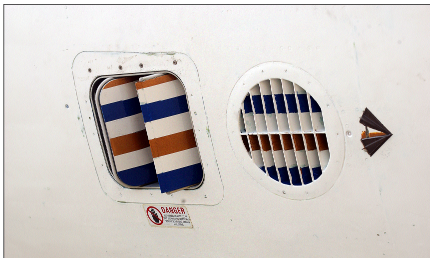
The thrust recovery outflow valve (TROV) redirects air exhausted from the cabin into the airstream, actually producing a slight forward-thrust vector.
