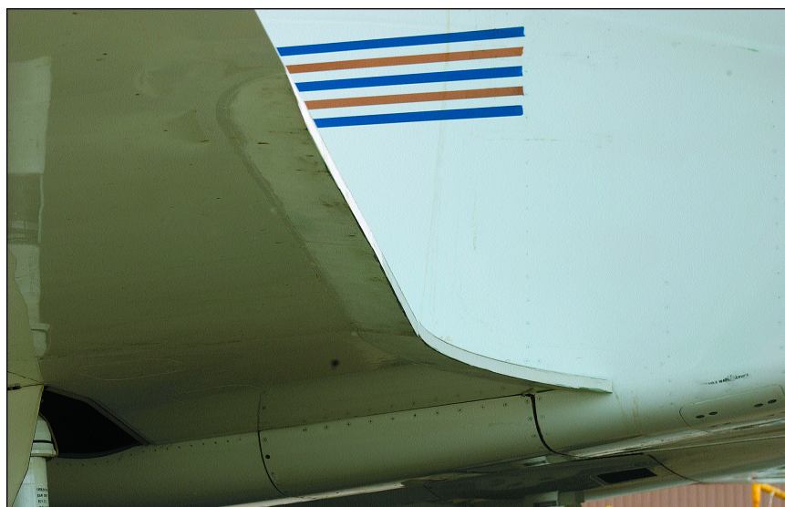
Trailing-edge contour wedges, on the inboard 30 percent of each wing, increase chord camber slightly, thereby creating a more elliptical lift distribution pattern.
