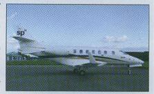
with 100-nm NBAA IFR reserves. Eight-passenger range will be 1,670 nm. Maximum takeoff weight will be 13,889 pounds, maximum fuel capacity will be 4,422 pounds and maximum payload will be 2,491 pounds. Pressurization is pegged at 8.4 psi, yielding a maximum cabin altitude of 8,000 feet.
