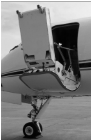
Some operators said that moisture intrusion into the main door seal was an ongoing problem.
