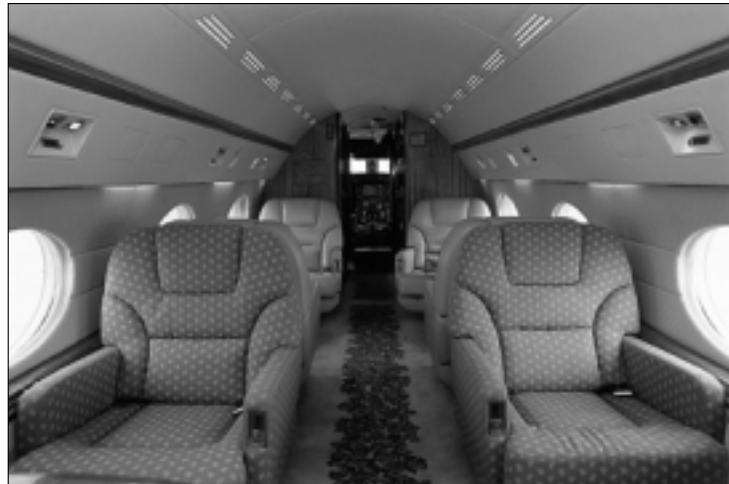
Cabin configurations vary, but almost all have three seating areas, with an aft galley and aft lavatory. About half of the operators said their aircraft have a second, forward crew lavatory.
