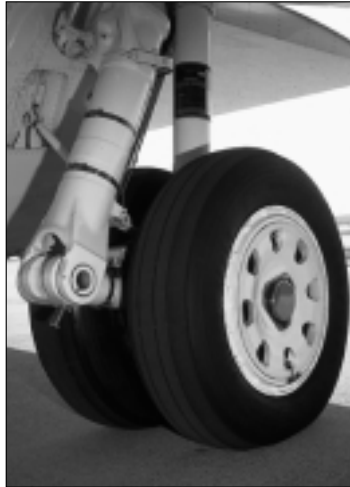
The G-IVSP's 66,000-pound max landing weight is made possible by more-robust rolling stock and wheel brakes, plus recalibrated main landing-gear strut damping.
