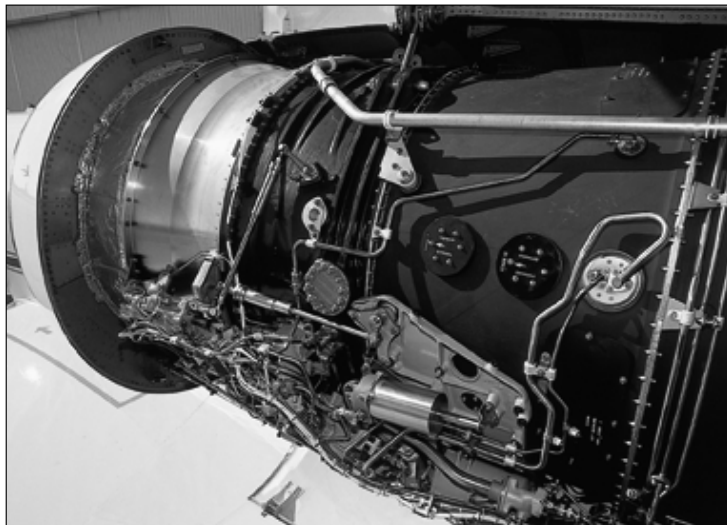
The Rolls-Royce Tay 611 engines received "A+" ratings from most operators, because of reliability and low maintenance requirements.
