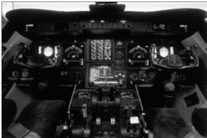
Operators said the SPZ-8000 avionics package (SPZ-8400 for serial number 1253 and subsequent) was quite reliable and capable. As shown in this photo, few opted to install the optional Honeywell-GEC Marconi HUD 2020.
