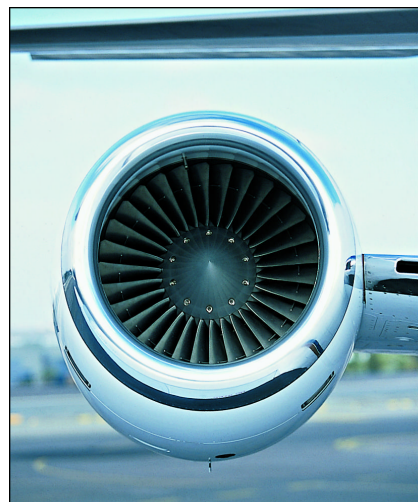
Honeywell TFE731-5BR engines are highly reliable, operators reported. Avoid the earlier -5AR engines. They don’t have enough takeoff or high-altitude thrust.
