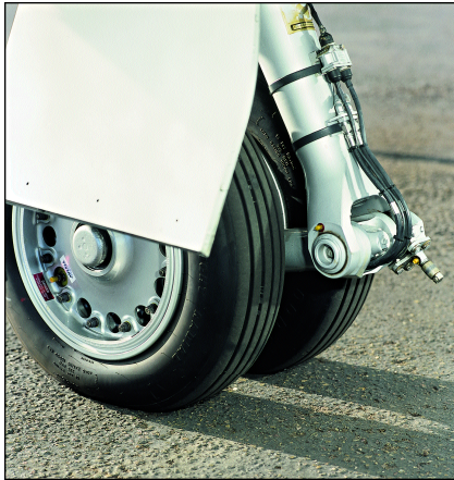
The trailing-link main landing gear makes for passenger-pleasing smooth touchdowns. Large rolling stock and wheel brakes provide excellent stopping power.
