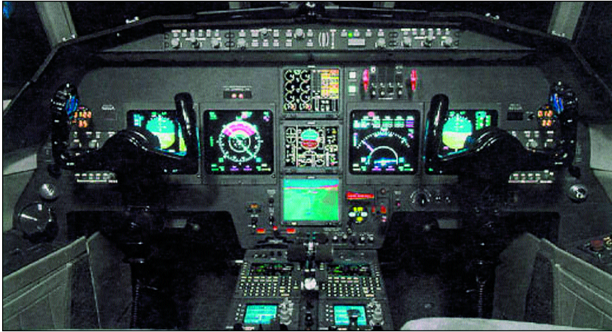
Some operators have chosen Rockwell Collins Pro Line IV avionics, giving their aircraft the appearance and functionality of a new Falcon 50EX.
