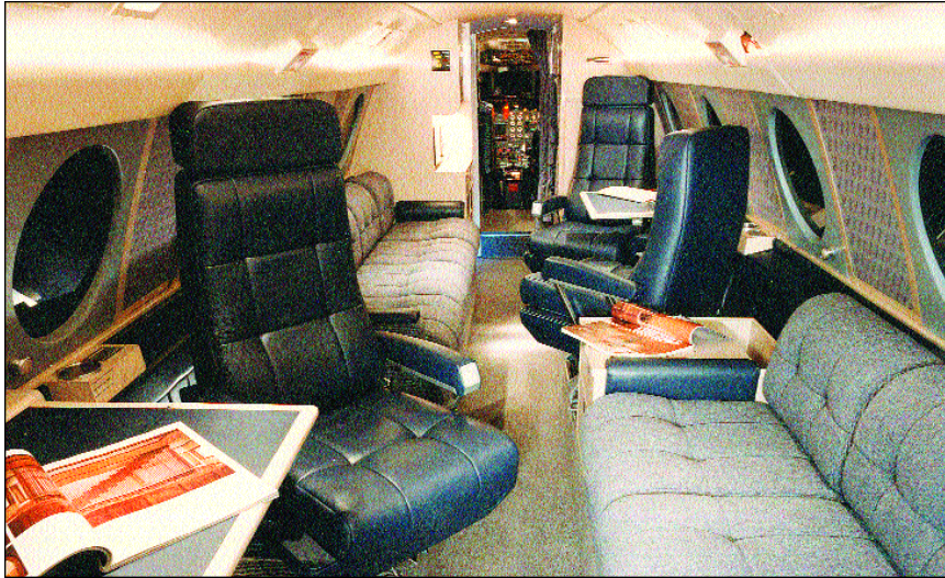
The interiors of most Falcon 20 aircraft are completely redone during the 12- to 16-week engine conversion process, thereby providing Falcon 50EX-class cabin comfort and passenger amenities. Garrett Aviation's Springfield, Ill., facility fitted the aircraft below with high-gloss wood-veneer cabinetry, a completely redone aft lavatory and a space-efficient forward galley with microwave oven.
