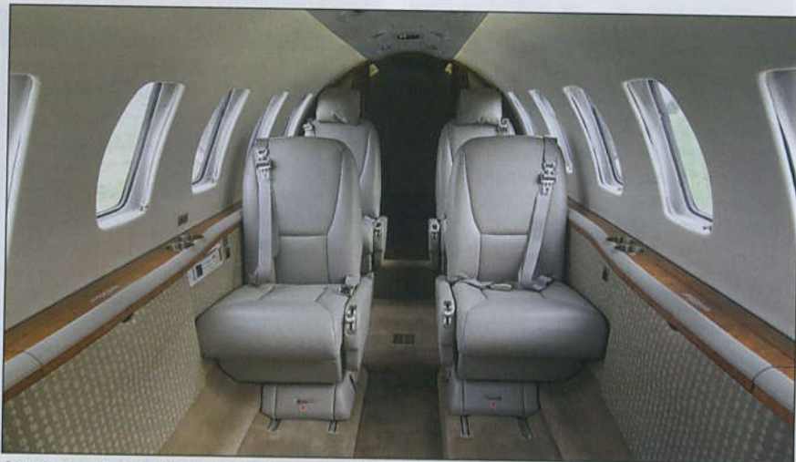
Standard cabin configuration remains center club, with two forward-facing single seats in the aft cabin and a right forward aft-facing seat (not shown). The overhead panel now features long-life LED wash lighting, and sidewall ledges have been fitted with a soft leather bull-nose cap.
