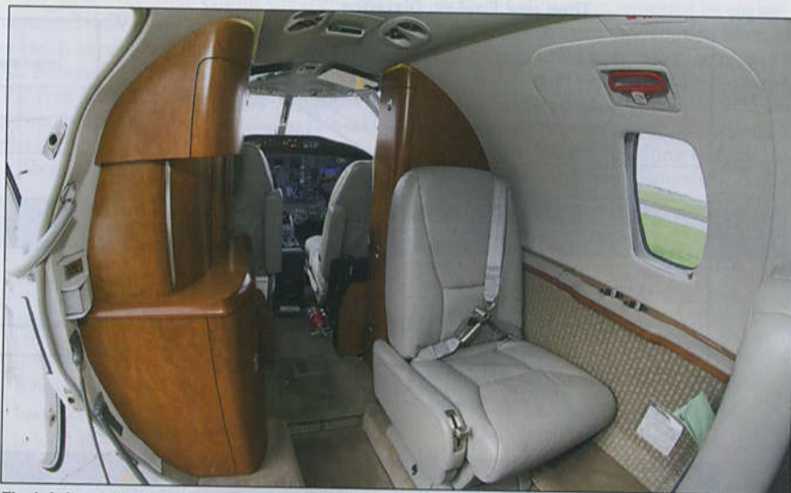
The left forward galley has been redesigned with softer contours. There is more storage capacity, and incandescent lights have been replaced with long-life low-heat LEDs. Just behind the copilot seat, there is a coat closet with a good sized compartment at the bottom to hold navigation publications or an EFB.
