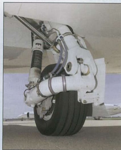
Trailing link main landing gear made its debut on the Encore. It works just as well on the Encore+ in providing consistently smooth touchdowns.
