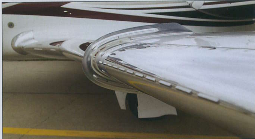
Bleed-air heating is used for wing anti-ice protection. Leading-edge boundary layer energizers, plus stall fences, minimize roll-off at the stall break.
