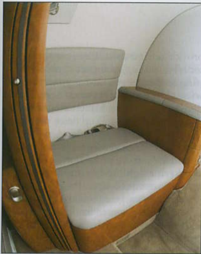
The aft lavatory, fully enclosed by a pair of solid pocket doors, has an internally serviced flush toilet. There is no wash basin, so plan on using moist sanitary wipes for post potty chore clean-up. The left side of the lavatory has an additional carry-on luggage compartment.
