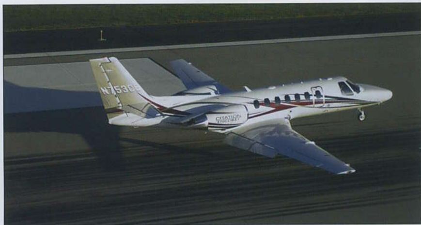
Short-field performance remains a strong suit of the Encore+. The aircraft has a 3,520-foot TOFL at MTOW and it needs less than 3,100 feet of runway for a 1,000-nm trip, assuming sea-level, standard-day conditions.
