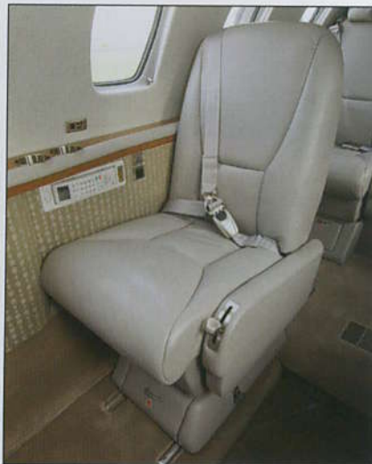
Each of the seats in the cabin adjusts in pitch, tilt, lateral track and yaw. The cabin now has standard AC power outlets for office equipment next to the left and right forward-facing seats in the center club section.
