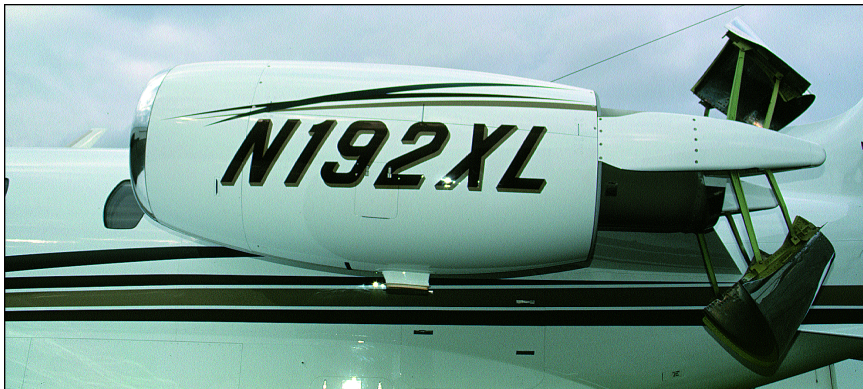
Cessna claims any thrust-reverser-induced tail shake should have no long-term effects on the empennage.
