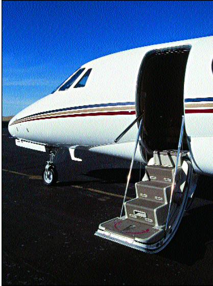
Lights in the Excel's airstair steps, along with a sturdy folding handrail, help passengers find solid footing and board with ease.
