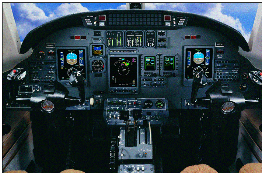
The 55-light master warning panel received some complaints — too busy and too many advisories.
