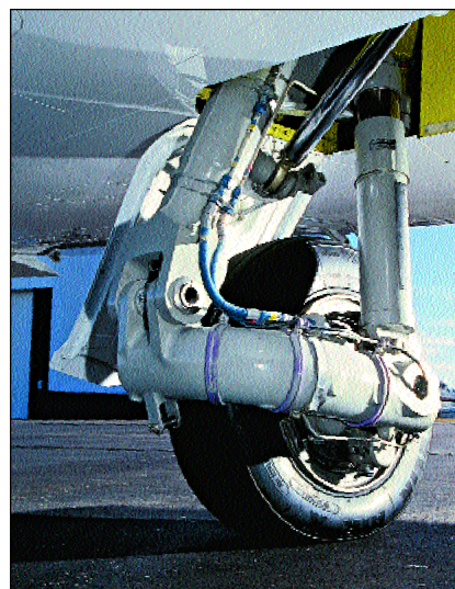
The Excel's trailing link, main landing gear received compliments.
