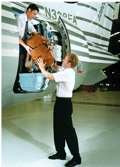
The Envoy 3's aft luggage bay, also accessible through a door in the aft cabin, has a 229-cubic-foot, 1,653-pound capacity.
