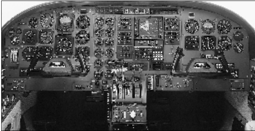
Cockpit design of the Conquest II wins praise from pilots for good layout, generous space. Visibility is good. Original equipment ARC avionics, including analog ARC 1000 flight control system, are weak points.
