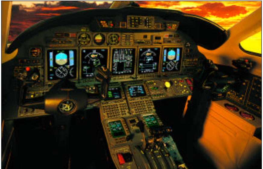
The Citation X's standard equipment now includes TCAS II, EGPWS and CVR. The Honeywell Primus 2000 avionics also has been upgraded.
