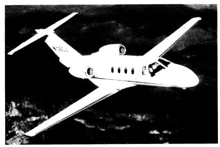
Cessna CitationJet is powered by two Williams-Rolls FJ44 turbofan engines. The aircraft is certified for single pilot operations.
