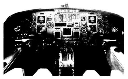
Standard Cessna Citation 2 avionics package includes a Sperry flight director/autopilot system including 4-in. conventional horizontal situation and attitude director indicators. Dual Collins VHF20A transceivers and VIR30A navigation systems are standard equipment, as is the Bendix RDR 1100 weather radar.
