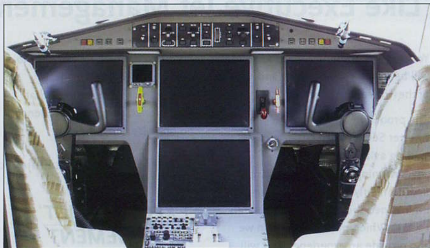
The Falcon 900EX EASy flight deck features four large LCDs, a graphical interface system and modular avionics architecture.
