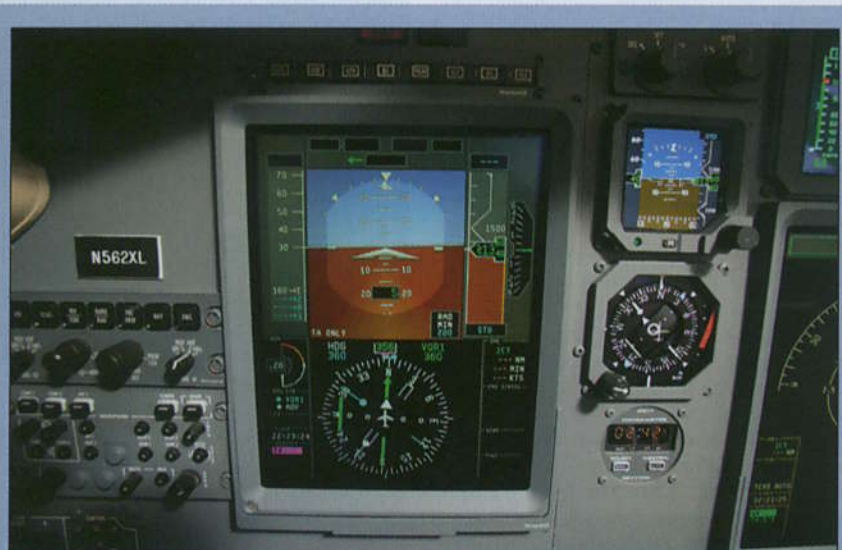
The standard, double-wide console accommodates a second FMS CDU and other options.
