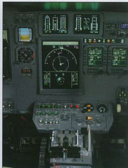
The centrally mounted MFD brings much-needed situational awareness improvements to the XLS.
