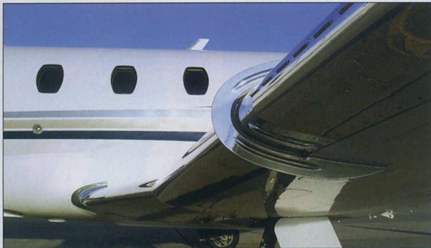
The XLS retains the Excel's leading-edge devices to enhance high angle of attack stability. But it still drops a wing during a full aerodynamic stall.
