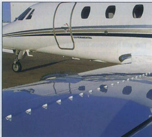
An array of 26 vortex generators on each wing helps prevent Mach-induced flow separation over the ailerons, especially important because the XLS cruises higher and faster at heavier weights than the Excel.
