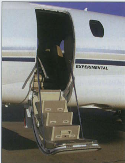
The sturdy airstair door has a robust handrail and tread lighting for safe boarding at night.
