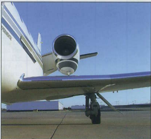
Wheel fairings under the XLS's wing reduced drag in climb and cruise.
