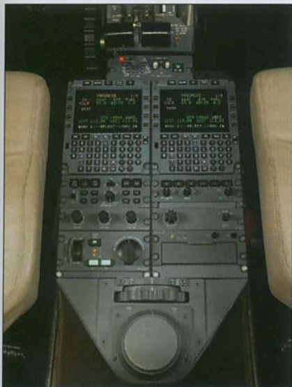
The standard, double-wide console accommodates a second FMS CDU and other options.
