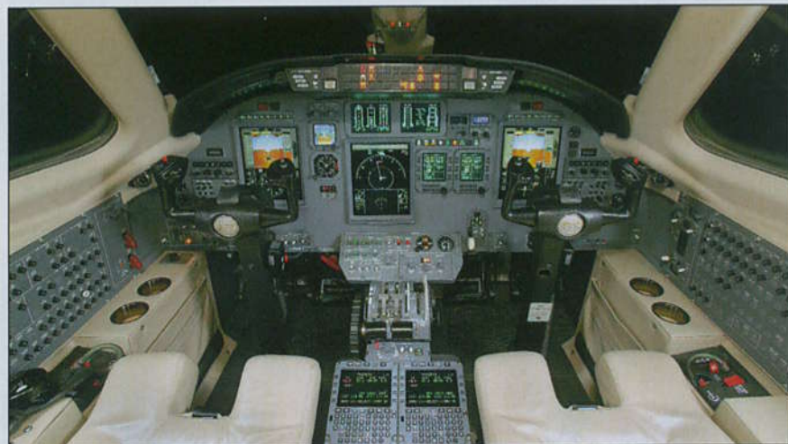
The instrument panel features the Primus 1000, with large-format flat-panel displays borrowed from the Primus Epic suite. But the rest of the panel is a virtual legacy from earlier 560 aircraft.
