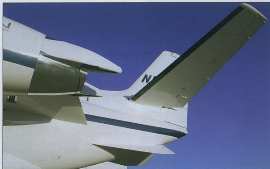
Thrust reversers are effective, but they do shake the horizontal tail at maximum output.
