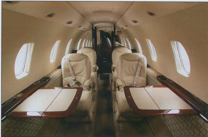
Outboard armrests have been eliminated and inboard armrests folded out of the way, affording passengers 4 more inches of usable width in the six main passenger chairs.
