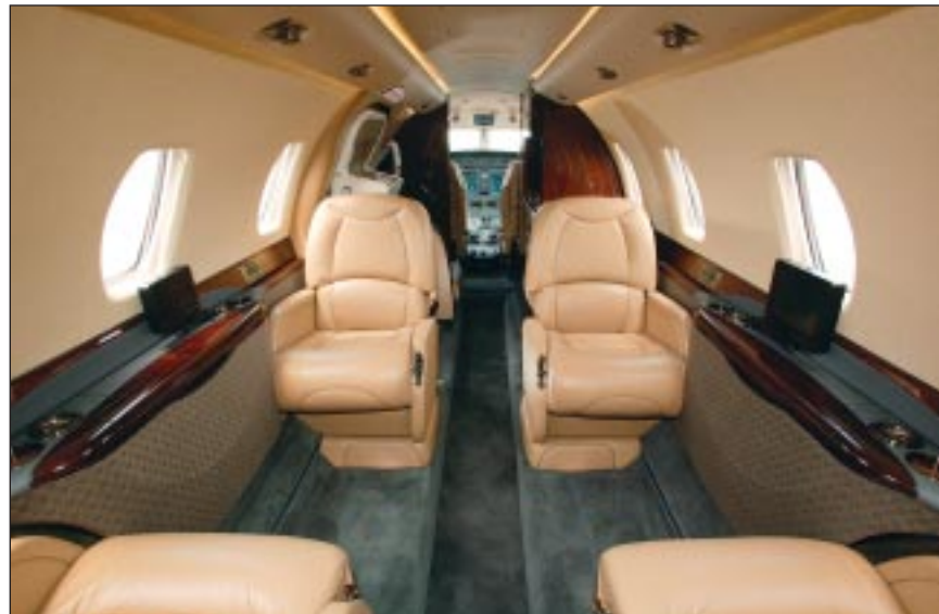
Maximum height in the 13-inch-wide, full-length dropped aisle was 5.7 feet.
