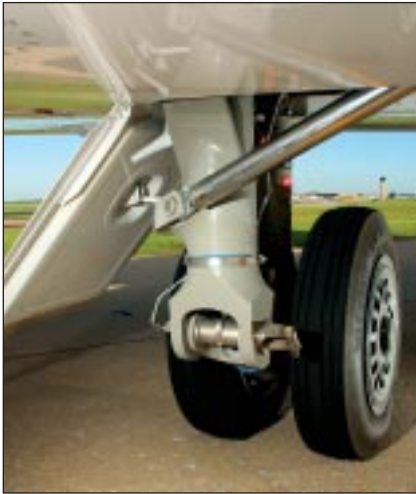
The main landing gear use a trailing link design for smooth landings and taxi.
