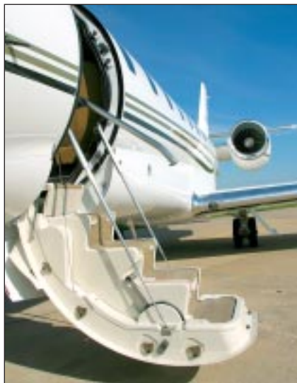
The airstair door has a solid feel and is nicely counterbalanced with springs.
