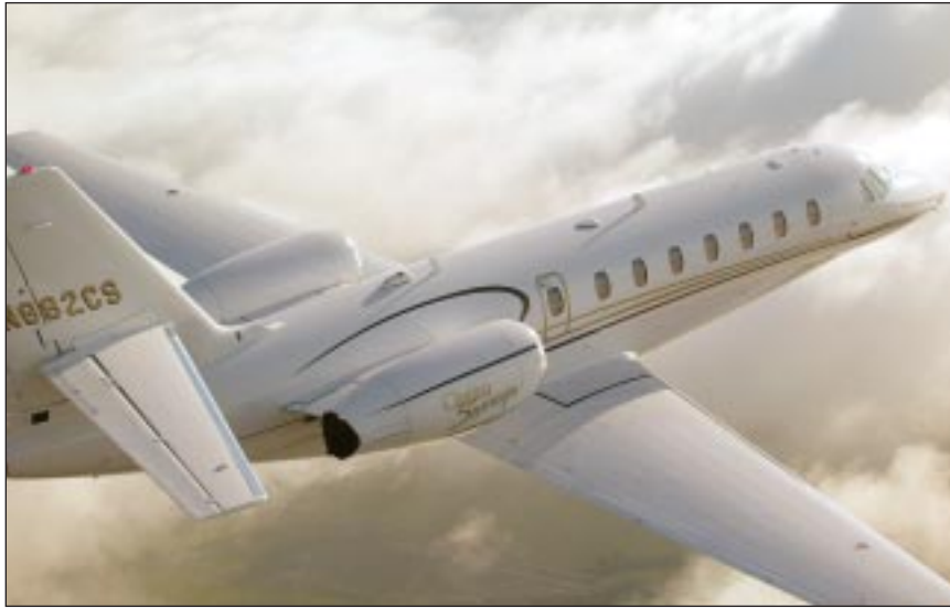
The Sovereign's 16-degree mildly swept wing leading edge and moderately super-critical airfoil shape enable it to cruise as fast as 0.796 Mach, or 454 KTAS at ISA-2°C, based upon our observations.
