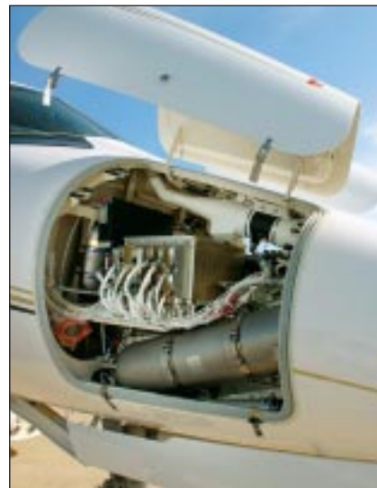
The Sovereign's nose section essentially is the same as that of the Citation X.
