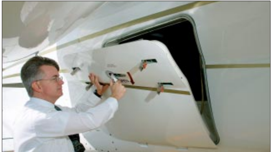
The Sovereign features a 100-cubic-foot, external aft baggage compartment.
