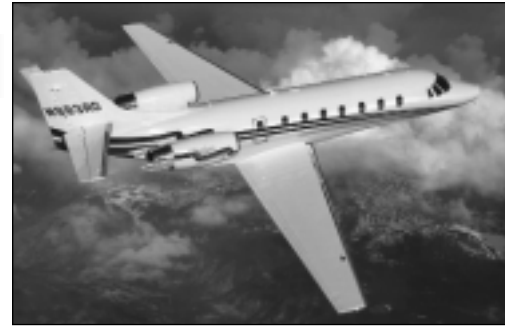
Cessna's new Sovereign has a super-critical airfoil.
