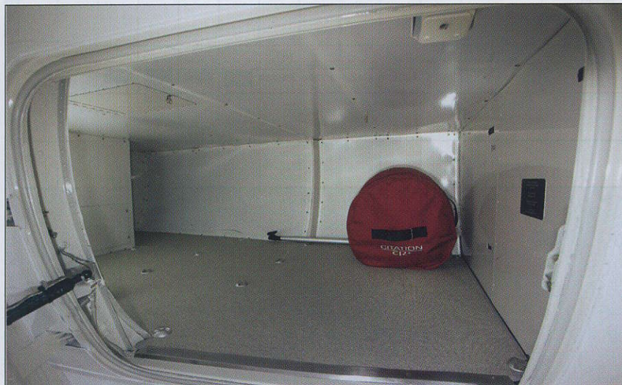
Both aircraft have generously sized, aft external baggage compartments, accessible through large doors below the left engines. The CJ2+, for instance, has a 50-cubic-foot, 500-pound capacity aft luggage compartment. There's another 15 cubic feet of space in the nose for luggage, plus additional room in the lavatory for carry-on items.
