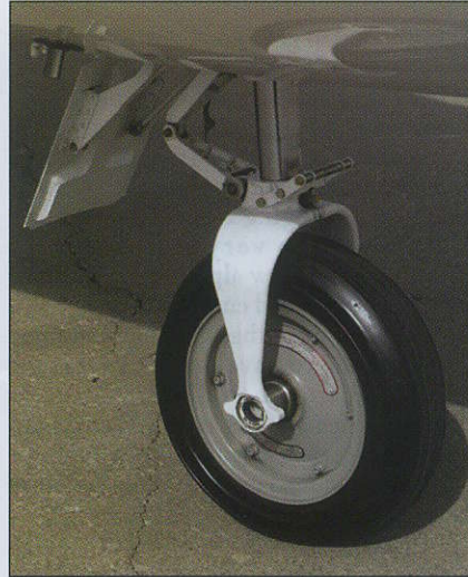
Nosewheel steering, in keeping with legacy short-wing Citation design practice, is actuated by means of bungees through the rudder pedals. It works just fine. Very tight turns require use of differential thrust and/or braking.
