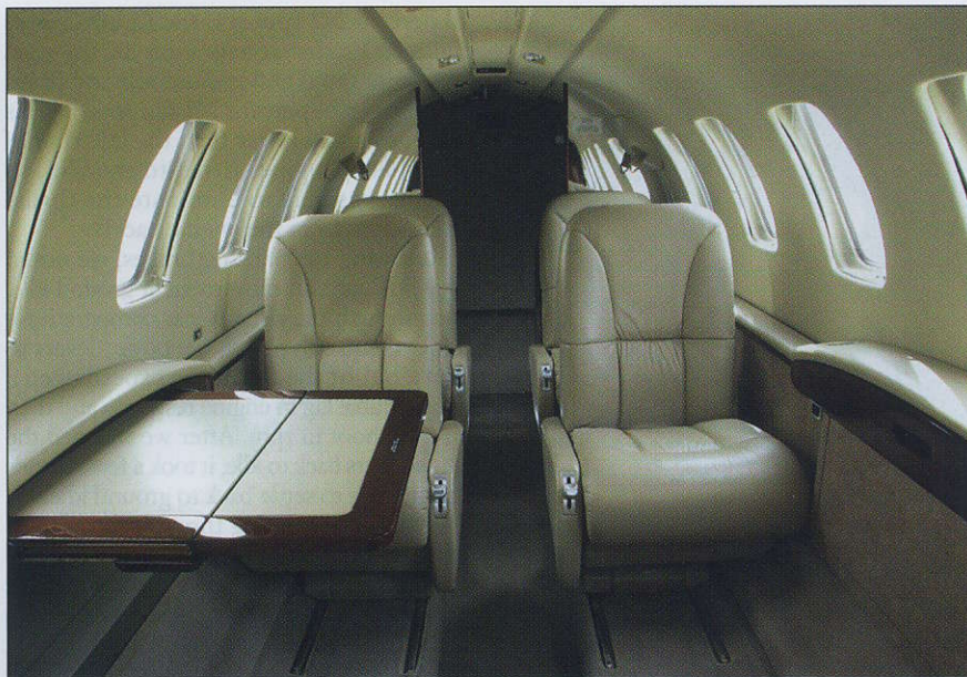
Cabins are equipped with long-life LED wash lights in the ceiling panels. Newly redesigned, manually operated window shades should offer improved reliability. Sturdy, foldout worktables are located between facing pairs of seats in the club section.
