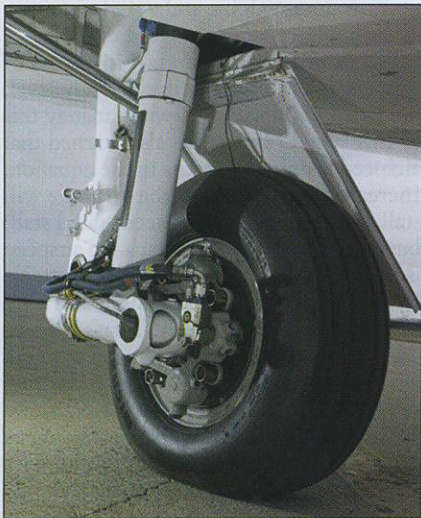
Long-travel, trailing-link main landing gear make for smooth landings and a comfortable ride on rough taxiways. The wheel brakes are improved, but we had difficulty modulating them smoothly during taxi.
