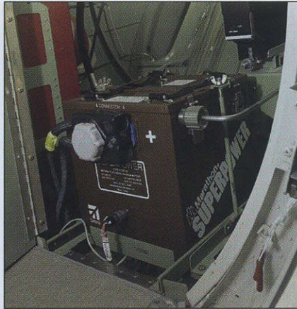
The standard battery is a nicad, but lead-acid batteries will be offered as no-cost options.
