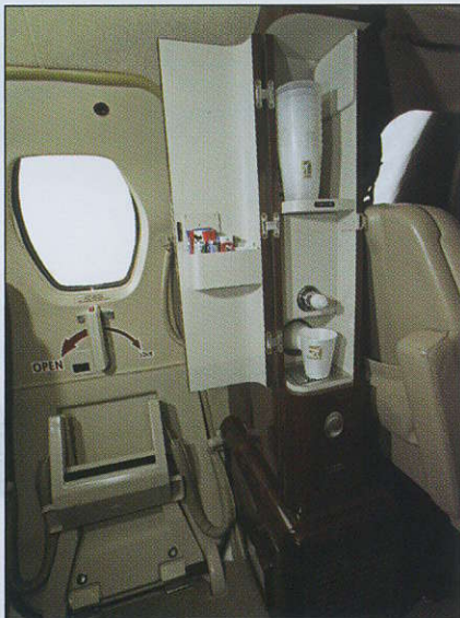
The compact, left-side galley accommodates a hot beverage container, ice chest, hot and cold beverage cups, beverage storage and refuse receptacle. The galley is ideal for short-range missions. Longer trips will require storing lunch boxes in the lav or in the cabin.
