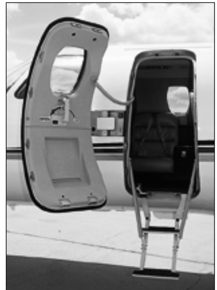
The main passenger door measures 50.7 inches high by 23.5 inches wide.
