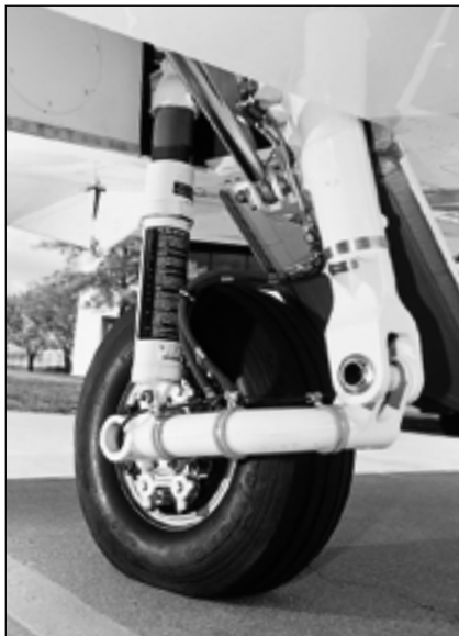
The CJ1 has trailing-link, main landing gear for soft landings and a smooth taxi ride.
