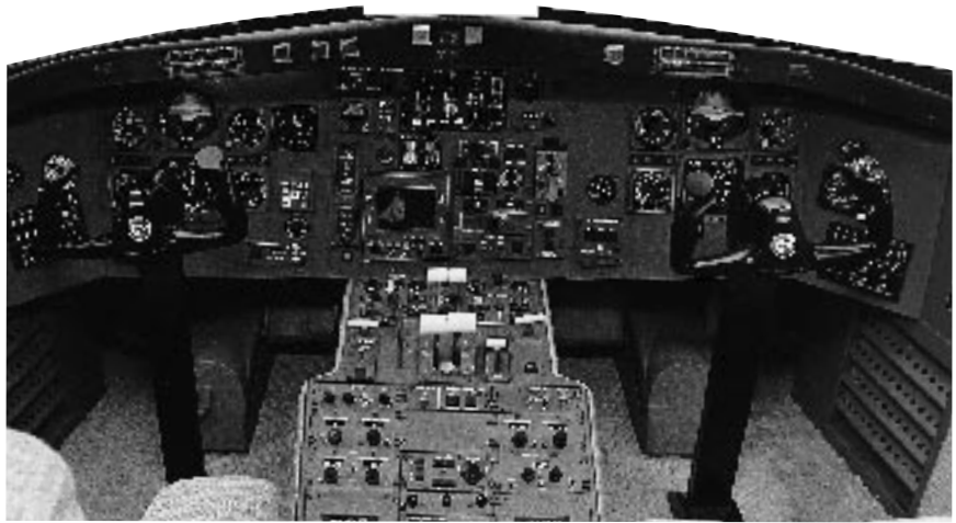
The original cockpit was sparsely equipped by today's standards. Popular options included INS, VLF-Omega and HF transceivers. What about RVSM? Plan on as much as $250,000 for equipment upgrades and certification.
