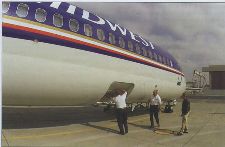
Almost all aluminum, the B-717's "double bubble" fuselage combines two cylindrical cross-sections joined at the floor for increased external baggage volume in the belly.
