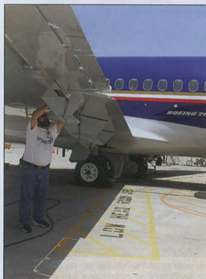
While both the leading edge slats and trailing flaps are hydraulic, the spoilers are fly-by-wire.
