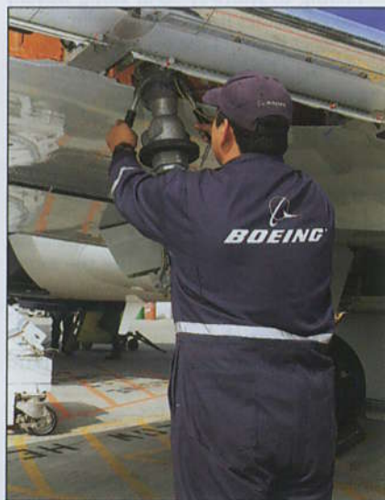
The single-point pressure refueling port is low enough to be accessible to most ground service personnel without them needing a ladder.
