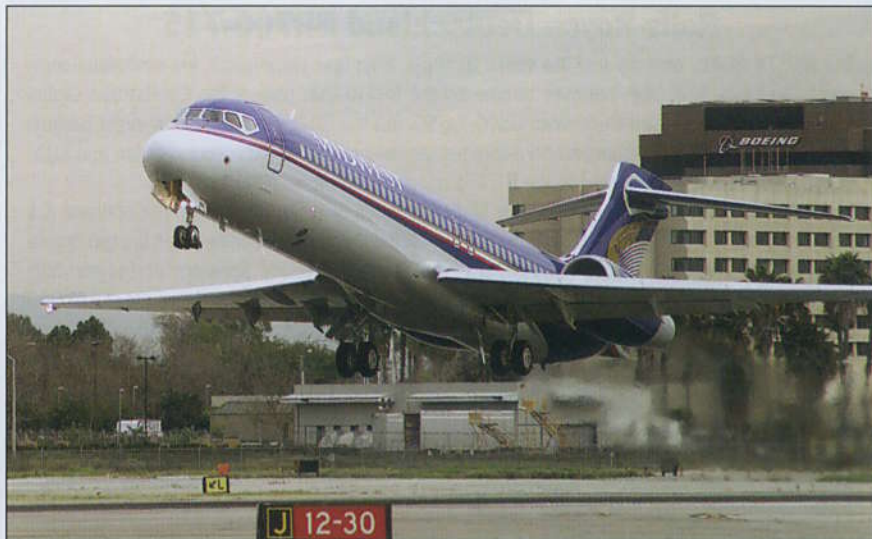
On our evaluation flight, the B-717 had a better thrust-to-weight ratio than a fully loaded Gulfstream 550.
