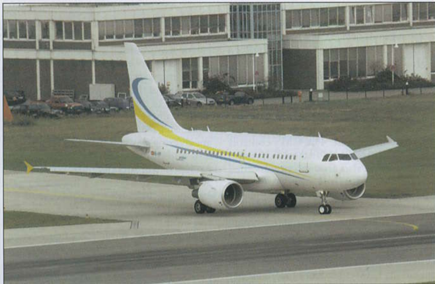
The windshield panes are glass/acrylic laminate panels and they're designed to be replaced in two hours.
