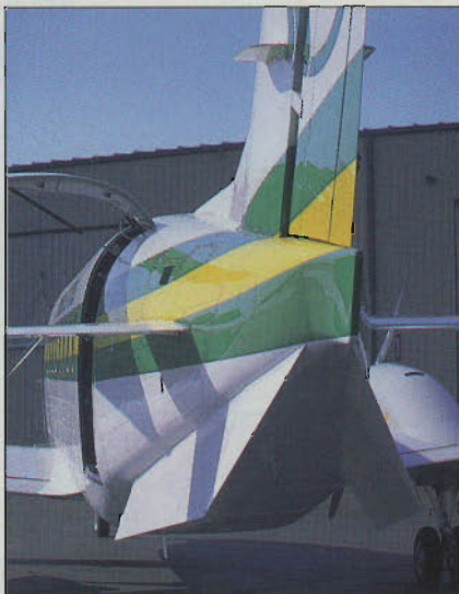
The 1900D has the familiar T-tail with its vertical taillets, one at either end of the horizontal tail. The wings are outfitted with an extension and winglets, increasing effective vertical tail surface.
