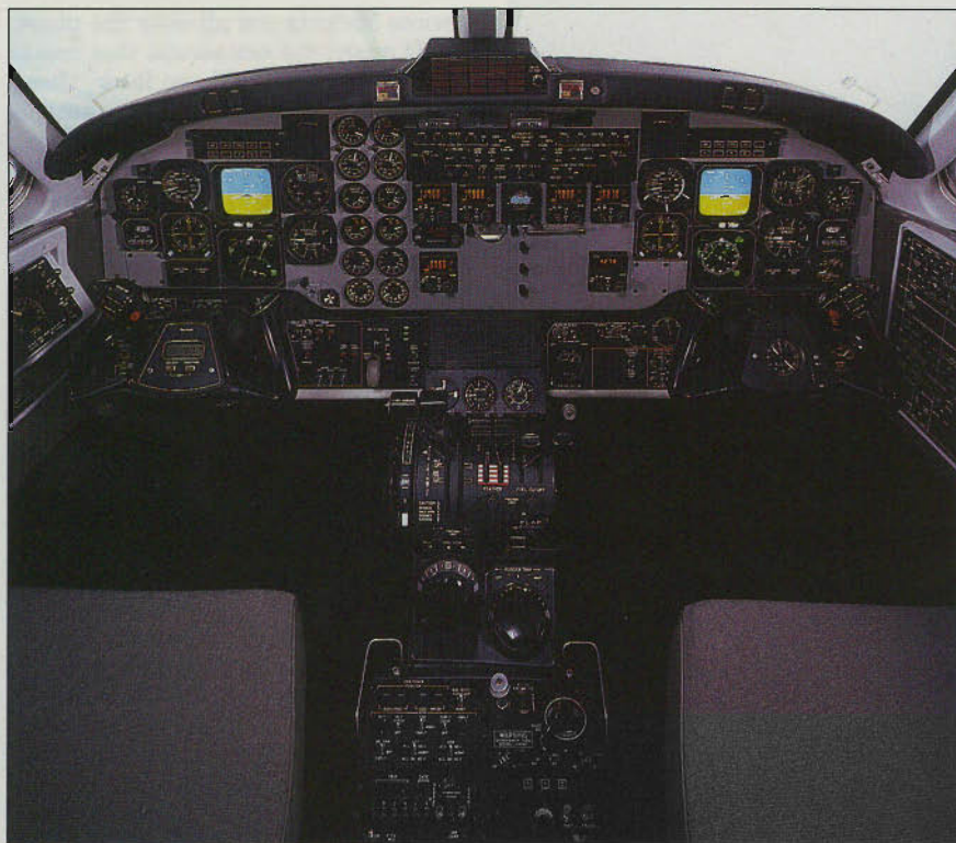
Standard avionics include dual four-inch Collins EFIS. The entrance door is larger than that of the 1900C, so boarding passengers do not have to duck through the portal.
